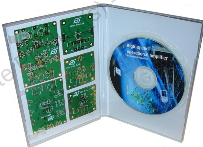
Figure 25: Evaluation kit for high-speed op-amps
